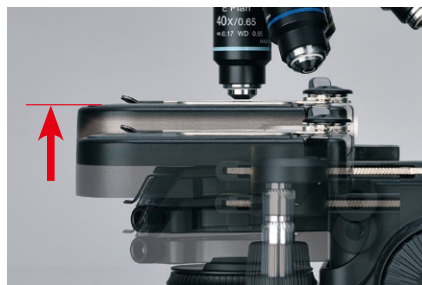
The stage does not rise above the set height.
