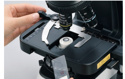
Easy-to-operate specimen holder
